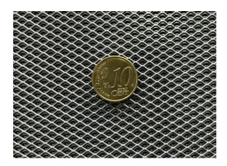
**Fine mesh** covers the range from a mesh length of 6.0 mm to 22.0 mm. Fine mesh also has good formability, as the mesh can be bent, refined or deep-drawn, for example. Both with a structured, three-dimensional surface and flat-rolled, fine mesh finds numerous applications. Here, too, the good economy and the high achievable free cross-sections are an advantage.
